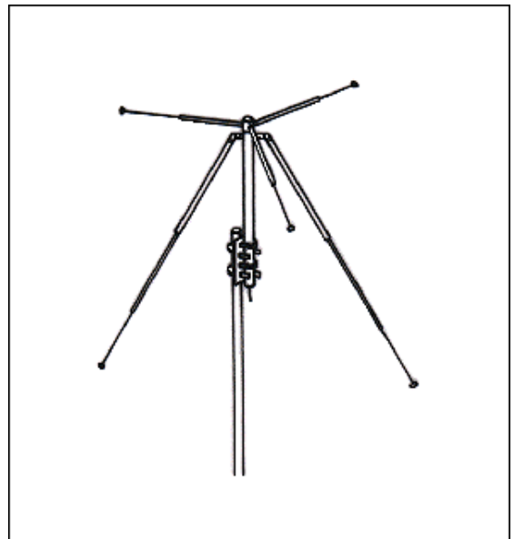
Figure 10.13 Mounting the completed antenna to the mast.
